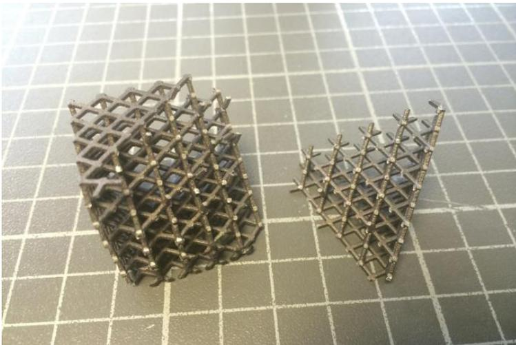
*Figure 2: Brittle failure mode of the lattice structure*
