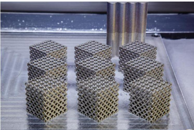
Figure 1: Sample parts with different volume fractions manufactured in Maraging Steel
